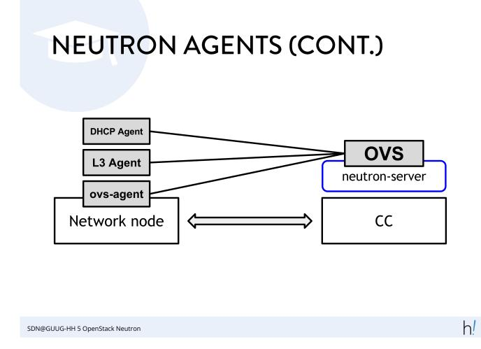
We have three specific agents running here: The ovs-agent, which is the agent that talks to the OpenVSwitch plugin on our cloud controller node The L3 agent, which allows client VMs to be accessible via official ("floating") IPs by setting appropriate iptables rules on the network node The DHCP agent, which supplies client VMs with internal IP addresses via DHCP Then, we have our computing nodes:
