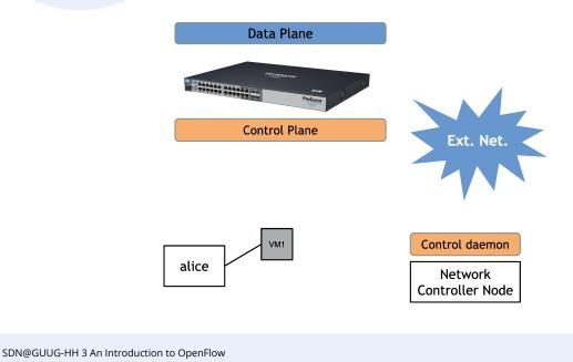
OpenFlow as a separate control plane running on its own host within the network. In such a scenario, the switch is downgraded to "iron only", i.e. the switch itself does not provide any actual management functionality, it doesn't even have to be a manageable switch.
