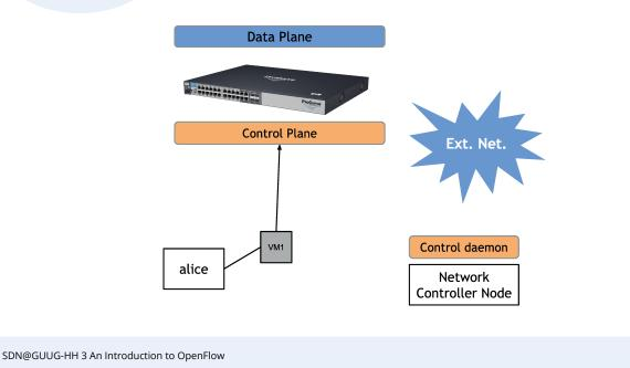
Here, the switch would receive the flows it needs from the SDN control daemon. So if a VM request hits the Switch forwarding plane, the Switch would ...
