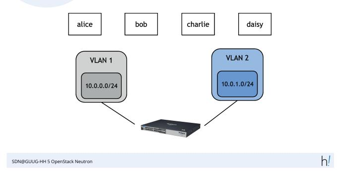
Our compute nodes use bridge interfaces and if a VM is to boot up in a certain VLAN ... a virtual interface is created on top of that bridge for the VLAN
