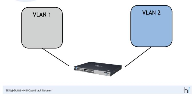
In conventional setups, additionally to switches, you will typically find VLANs, which are used for security reasons and to separate individual customers from each other.
