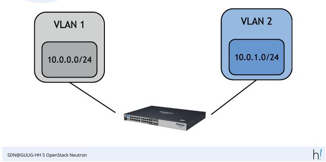
So every VLAN is assigned statically to a customer and will typically contain exactly one VLAN network (as it used to be in the good old days where everything was on iron, as just explained, too)
