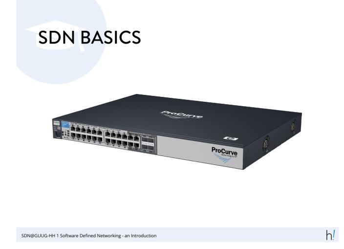
Let's jump back to the switch for a second. Within a switch, you will typically have different parts responsible for doing different things. A switch needs to do two things: send and receive data coordinate data it receives and it sends out
