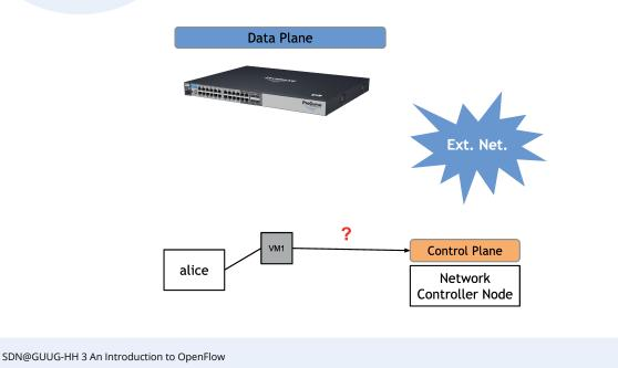
Because in a setup like this, where a VM is running and gets its flow information from the separate, OpenFlow compatible forwarding plane, a request is simply going the route it receives from the forwarding plane.
